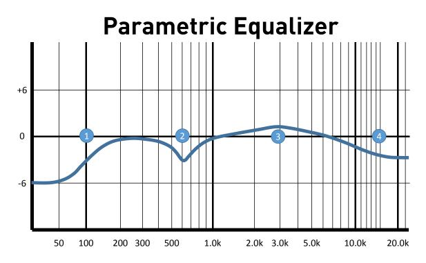
Using the Neuro App or USB Editor, Band 1 (Low Shelf) can optionally be configured as a high pass filter, and Band 2 (High Shelf) can optionally be configured as a low pass filter.
