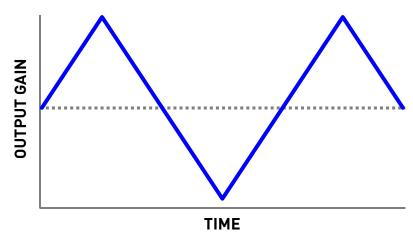
The blue line in the graph is known as the LFO. It changes the level of the output signal over time.
