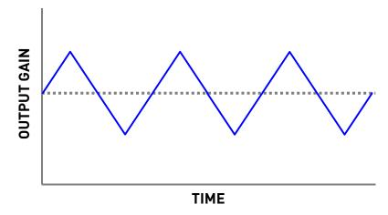
Finally, the shape of the LFO can be changed to give the tremolo effect a different character.
