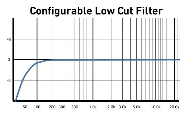
The Parametric EQ and the Low Cut filter are configurable using the Neuro Hub or USB Editor software. By default, the parametric EQ is disabled (flat), and the Low Cut filter is set to 10 Hz.
