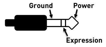
Expression pedals with TS (Tip Sleeve) plugs will not work correctly with the Vertigo.
