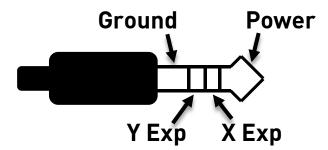
Third party expression pedals can be used as well, as long as they have a TRS (Tip Ring Sleeve) plug with power on the tip, expression (the wiper of the potentiometer) on the ring, and ground on the sleeve, as seen in the diagram below.
