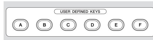
When the device is in the default state, USER DEFINED KEYS (page 14) are configured as "Direct Scene Recall" keys. You can save a Scene by pressing and holding down one of the USER DEFINED KEYS, and recall a Scene by pressing one of the USER DEFINED KEYS.
