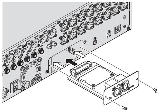
Make sure the sides of the NY card with the guide rails of the device you are installing it in.
