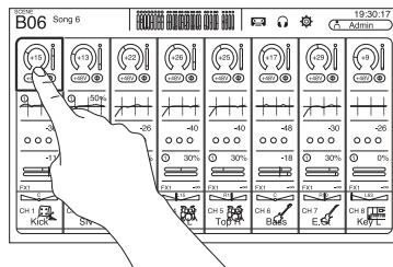
You can switch between the FADER section and the CH STRIP section by pressing the home key while the OVERVIEW screen is displayed.
