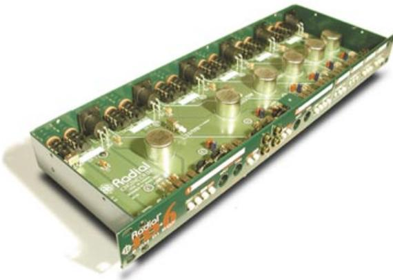
The Radial JD6 is a six channel, rackmount direct box designed for keyboards and electronic drums for both live and recording environments. The JD6 is equipped with premium Jensen transformers for maximum headroom and low phase distortion to render the most natural sound. This is of particular importance for digital pianos that are both extremely dynamic and have tremendous harmonic content.
