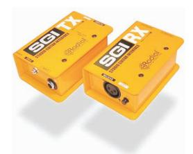
Radial SGI Studio Guitar Interface is a transmit (SGI-TX) and receive (SGI-RX) pair of modules that allows a guitar signal to travel across 500 feet of balanced cable to a distant amplifier. The SGI is a unity gain device that features 100% discreet Class-A circuitry for great sound and transformer isolation to eliminate ground loops.
