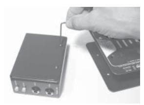
When tightening, make sure you get a nice snug fit but do not overtighten as this will only make removing the device more difficult later on.
