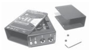
Install the smaller J-Rak shells. Be careful not to strip the screws or pem-nuts. Note that the XLR connection is always on the bottom.
