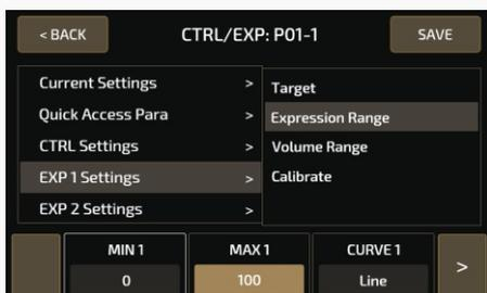
In the selection panel, MIN X (X standing for 1-4 controllable targets) represents the lowest range value. This is the value the pedal will have when pushed all the way up. MAX X represents the highest range value, when the pedal is pushed all the way down. CURVE X represents the curve line the pedal will follow when pushed from all the way up to all the way down.
