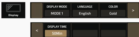
Use DISPLAY MODE to switch two display modes in Main Display screen. Mode 1 stresses patch number, and Mode 2 stresses patch name. Default is set to Mode 1.
