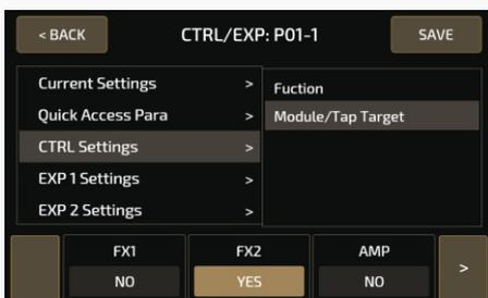
The 9 Ampero One effects modules are listed in the panel, with yes and no below each module to show if the CTRL footswitch is activated or not. In the example image above, FX1 and FX2 are controlled by the CTRL footswitch, whereas the AMP module is not. Slide (or use Main Knob) to change between yes/no, and press the arrows on the right/left to scroll through the modules.
