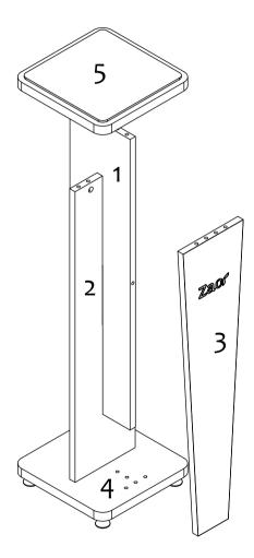
Here you have an exploded view of the whole stand and how it is supposed to come together. We use high quality furniture assembly components from renowned EU manufacturers. Please, never use force. These parts should come together easily, in case of doubt check the manual again or contact support.
