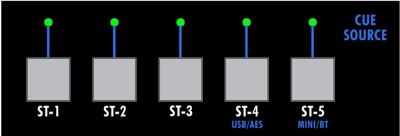
Five (5) input source selectors provide a choice of seven (7) different audio sources to feed the selected set of monitors. Each input source is buffered with an API 2510 op-amp. Only one source can be selected at a time.
