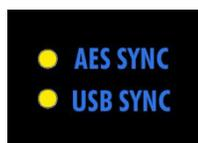
Yellow **AES SYNC** and **USB SYNC** LED indicators will illuminate when the MC531 is locked to valid **AES** and/or **USB** digital input sources.
