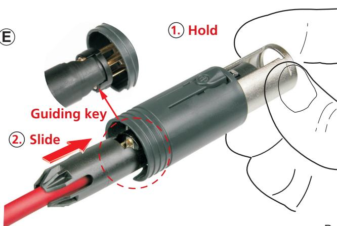
Put chuck onto the cable and slide insert & chuck into the housing.
