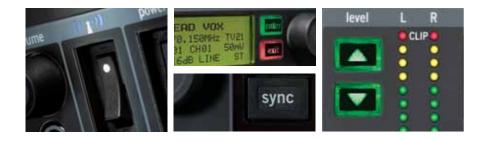
**Left:** RF mute switch prevents RF transmission during setup
