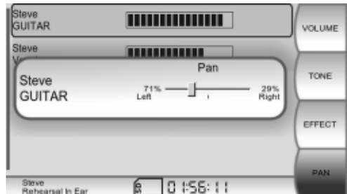
For a stereo signal, the panorama turns into a BALANCE control. Each individual channel of a stereo signal is routed 100% to the left or right by default. BALANCE allows you to move the stereo image to either side.
