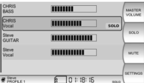
A yellow SOLO indicator will appear on the channels that are in SOLO mode. Additionally, a SOLO indicator will appear in the status bar. Push the SOLO soft key again to clear the channel SOLO. Pushing and holding the SOLO button for more than three seconds clears SOLO for all channels.
