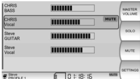
A red MUTE indicator will appear on the channels that are in MUTE mode. Additionally, a MUTE indicator will appear in the status bar. Push the MUTE soft key again to clear the channel MUTE. Pushing and holding the MUTE button for more than three seconds clears MUTE for all channels.
