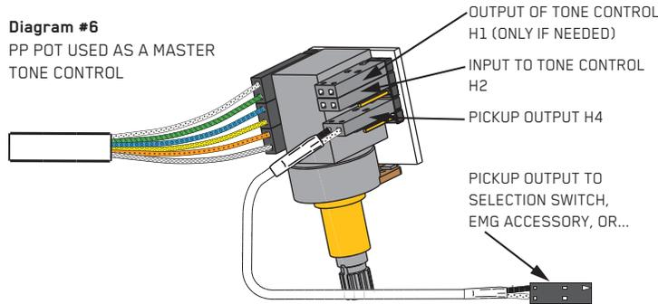
Diagram #6 uses the 25K Tone control independently of the pickup output. By taking the output of the pickup from Position H4, the control is now available to use as a Master Tone with H1 and H2 being the input and/or output of the Tone control. H1 and H2 positions are interchangeable. Position H4, the output of the pickup, would typically go to a selection switch or a pan-pot.
