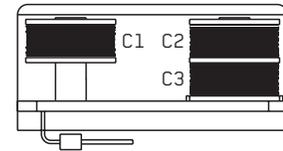
In Dual-coil mode, coils C1 and C2 are active.
