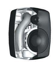
**Figure 3**: The curved reflex tube provides low distortion and excellent bass extention.
