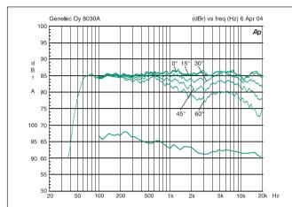
**Figure 3**: The upper curve group shows the horizontal directivity characteristics of the 8030A measured at 1 m. The lower curve shows the systems power response.
